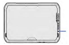
**NOTE -** Do not press the Power button repeatedly; do not hold the Power button for four seconds or longer.
