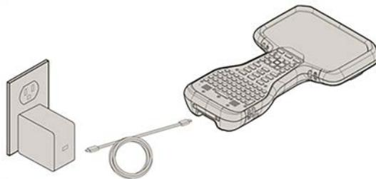
The internal Ranger 5 data collector batteries will charge first. When the internal batteries are fully charged, the optional Li-35 accessory battery pack, if installed, will charge.
