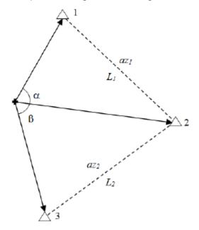
with: 2 observed control points 1 and 2 (coordinate values X<sub>1</sub>, Y<sub>1</sub>, X<sub>2</sub>, Y<sub>2</sub>)
