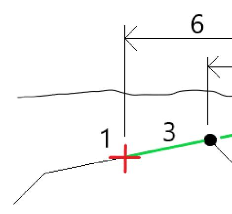
Stake details for the secondary road reported in the **Confirm staked deltas** screen include V.Dist to road (4), Horizontal construction offset (calculated) (5) and Distance to alignment (6).
