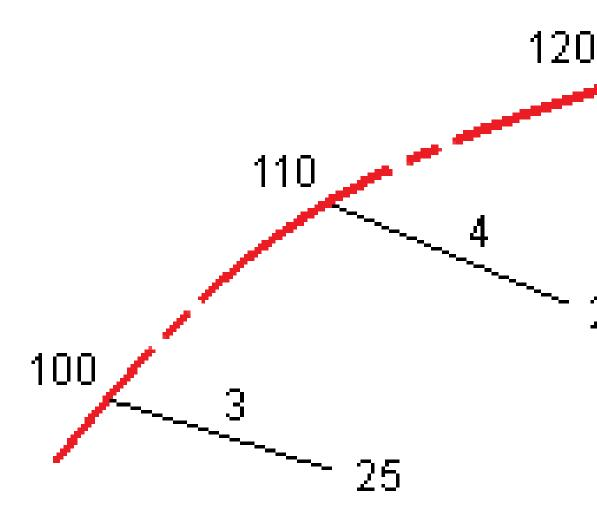
However, if the deflection angle of the 3D string compared to that of the associated 6D string is greater than 30 minutes, the geometry of the associated 6D string will be ignored and the coordinates will be computed by linear interpolation instead. This is to avoid unexpected behavior when there is an acute change in direction in the 3D string for features such as slip lanes, bus bays, and so on.
