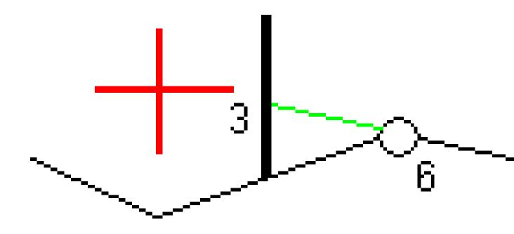
**NOTE** – For points with zero offset, you cannot apply horizontal construction offsets at the slope value of the previous line.
