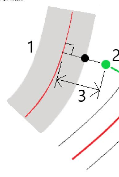
The cross section for the secondary road (1) at the computed station is displayed along with the position selected to stake on the primary road (2). Tap the line (3) preceding the position you want to stake on the secondary road:
