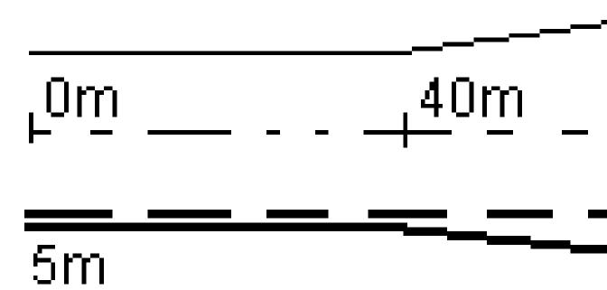
If you select an offset/string that has an offset value of 5 m, the offset value updates to follow the solid line for subsequent stations. In this example, the offset changes from 5 m to 8 m between stations 40 m and 100 m and then is maintained at 8 m for subsequent stations.
