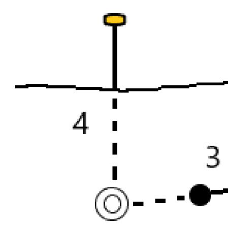
• **Perp Dist** (perpendicular distance) to the surface between the two strings.
