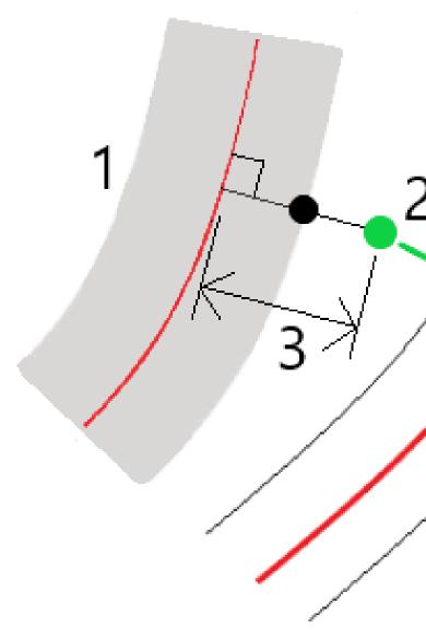
b. The cross section for the secondary road (1) at the computed station is displayed along with the position selected to stake on the primary road (2). Tap the line (3) preceding the position you want to stake on the secondary road:
