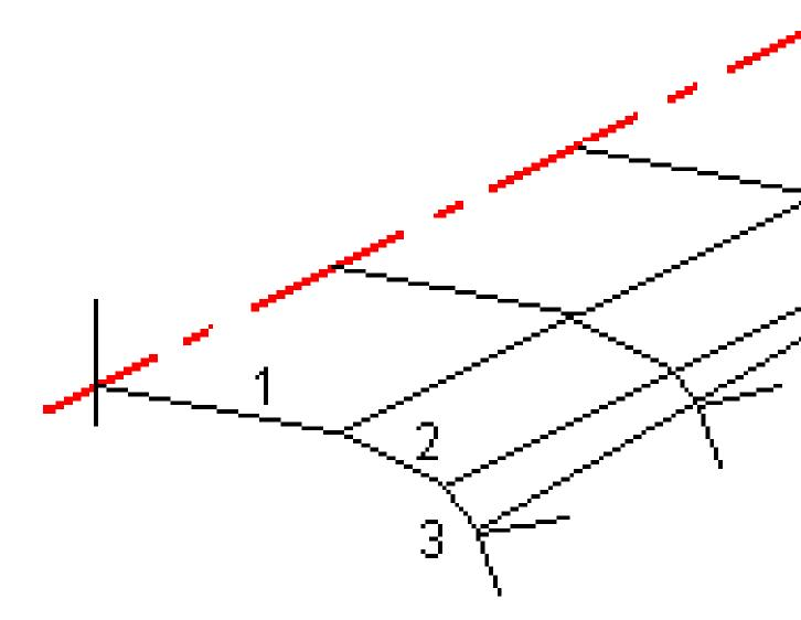
By adding strings defined with a zero offset, you can further control the interpolation process to best represent the road design.
