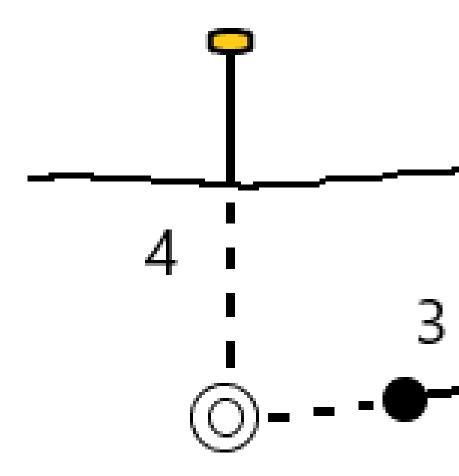
• **Perp Dist** (perpendicular distance) to the surface between the two strings.
