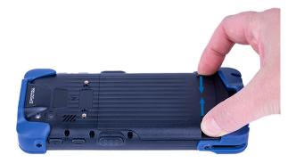
2. Push the battery forward and lift to remove it.
