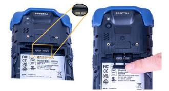
The card holder can hold two nanoSIM cards, or one nanoSIM card and one microSD card at a time. Insert your cards as needed, as follows:
