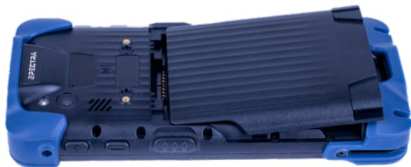
2. Press and hold the two plastic clips at the end of the battery, then push the battery forward and down into the battery compartment.
